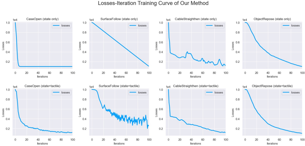
Figure 7: Training loss curves of trajectory optimization method for four contact-rich manipulation tasks. The top row shows the training with state-only observations and the bottom row shows the training with state+tactile observations.
